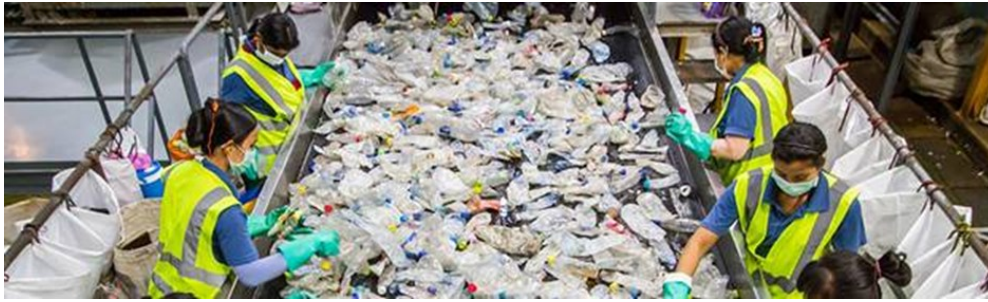
Figure 4 Sorting process of PET bottle wastes [12]
